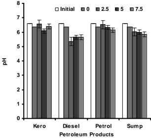
Fig. 2: Variations in pH of samples treated withvarious petroleum products
